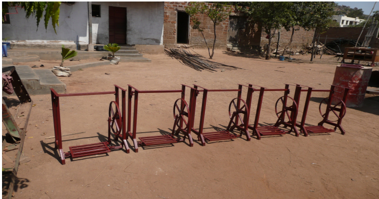
Treadles being produced in Mwanza City by Joshua. They are both robust and well designed using jigs and formwork. Over 300 treadles a year are needed for the project, a valuable income to local metal fabricators like Joshua.
